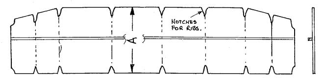
The completed wing must not exceed 5.0 inch chord. Lets assume that Dimension A is important. the L.E. and T.E. are 1/16 sq. (medium). Lightly sanded assume .06 in.
